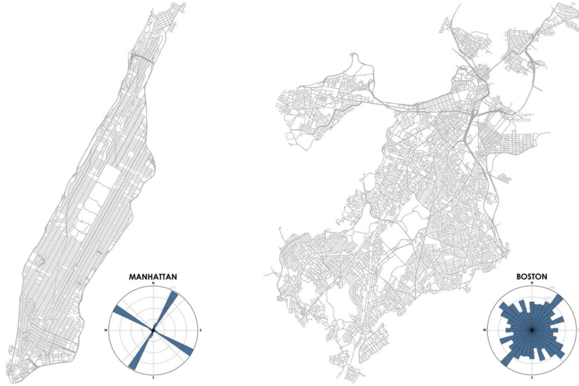
Figure 2.7: Two examples for the polar distributions of street patterns. Manhattan, NY, USA (left) has a higher street orientation-order \phi than Boston, MA, USA (right). Manhattan’s street network is almost exclusively distributed in four cardinal directions, i.e. two-dimensional, except for isolated symmetry breaks. Boston, on the other hand, represents one of the least grid-like cities in the USA. [Boe19b, Figure 3]
