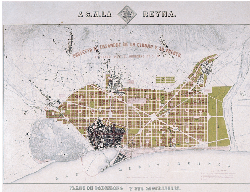
Figure 2.2: The approved Plànol del projecte Cerdà for Barcelona from the year 1859. Building footprints are shown in red and green space was reserved as public, green space. [Cer59]
