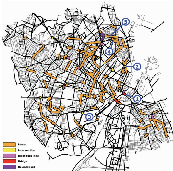
Figure 8. Overview map of top 105 gaps by class: streets in orange, intersections in yellow, bridges in red, right-turn lanes in pink, roundabouts in violet. Errors are shown in Appendix B. Numbered blue circles indicate the top 5 gaps (see Fig. 9 for detail plots). The street network is shown in grey, the bicycle network in black. See https://fixbike.net for an interactive version.
