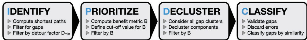
Figure 2. Steps in the IPDC procedure. Gaps are first identified via shortest paths, discarding parallel paths using a minimum detour factor D_{\min} . Gaps are then prioritized via a gap closure benefit metric, in the simplest case based on betweenness centrality. Resulting gaps can overlap (cluster) and need to be declustered. Finally, gaps are compared with existing infrastructure, validated or discarded, and classified.
